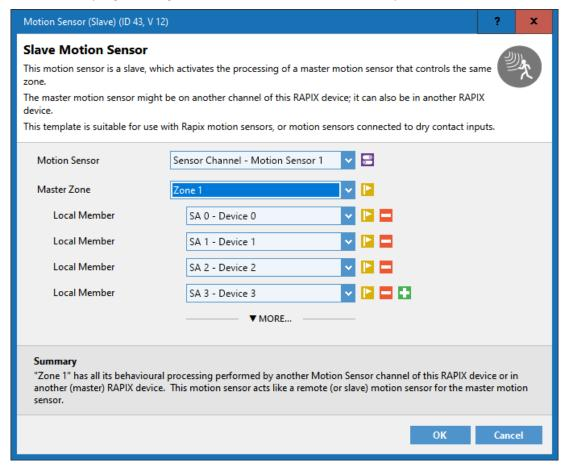
If Master and Slave sensors are on different DALI lines, a Zone Controller is needed to link the lines together and allow the sensors to work with each other.
