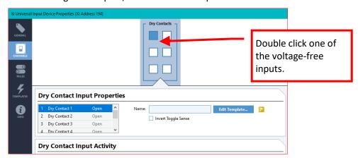
The settings page will appear allowing the setup of the sensor:
