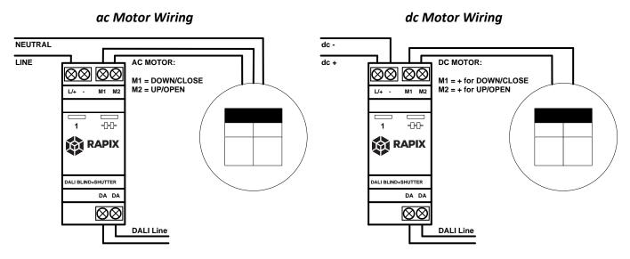
For ac motors, do not connect neutral to the relay unit.
