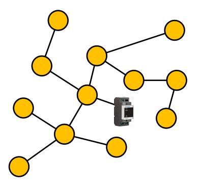
Compared to a power supply at one end of a line: lower voltage drop to the ends.
